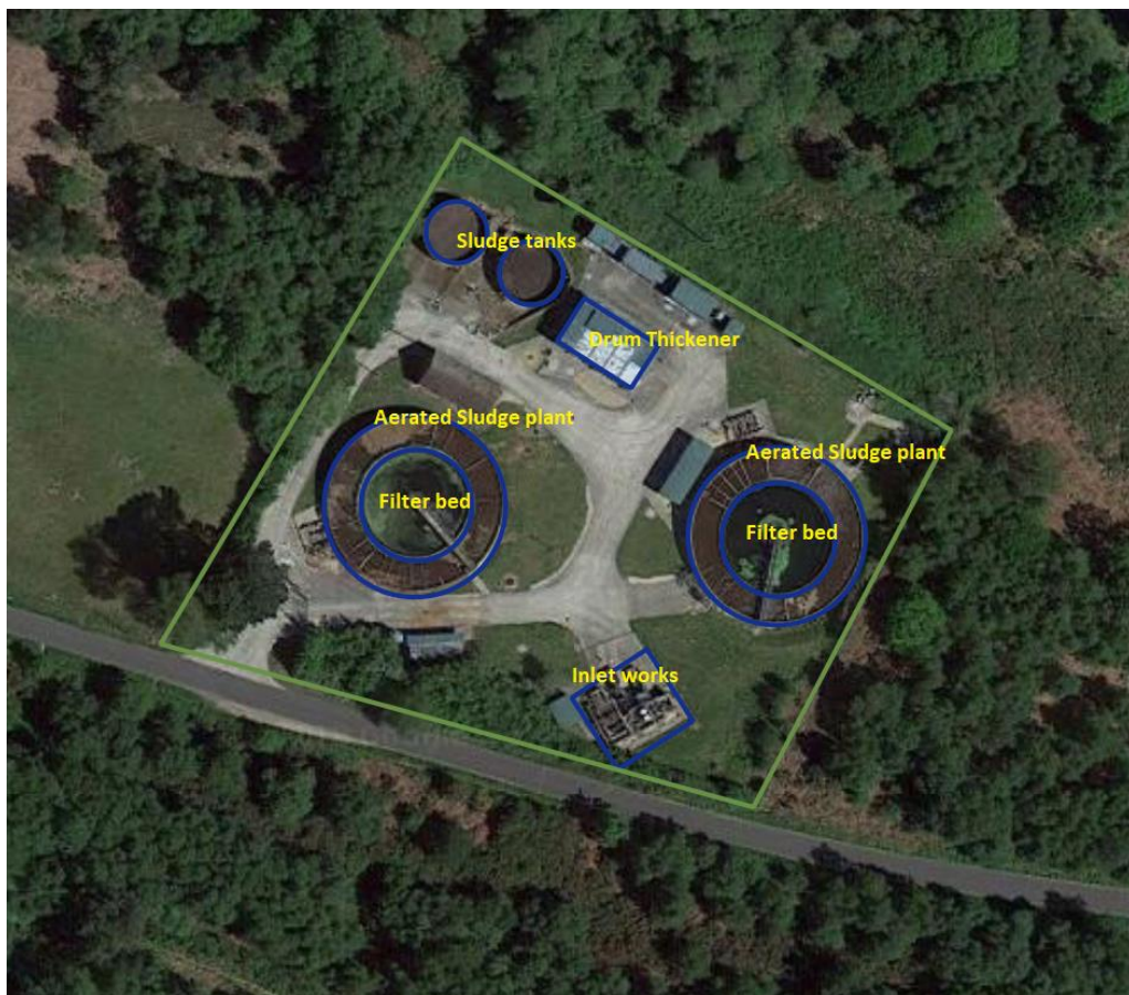
Figure 2 – Location of assets within Wool Sewage Treatment Works
